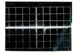
Differentiated Sync at Terminal AH 5 Volts/cm Sweep: 10 microsec/cm
