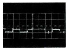
Red Signal at Kinescope Pin #4 100 Volts/CM Zero Volts DC at Bottom Line of Graticle
