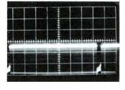
Blanking at Kinescope Grid #1 20 Volts/cm Sweep: 2 msec/sec
