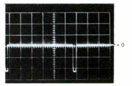
Burst Key Pulse at Terminal AG 5 Volts/cm
