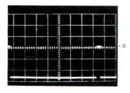
Vertical Drive at Terminal L 5 Volts/cm Sweep: 2 msec/cm
