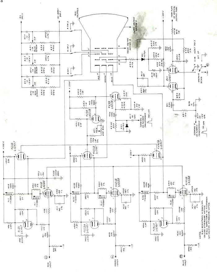
VIDEO AMPLIFIERS AND KINESCOPE CIRCUITRY (452068C, Sheet 10 of 10)
