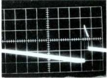
Vertical Output at Pin 2 of 5V1 200 Volts/cm Sweep: 2 msec/cm
