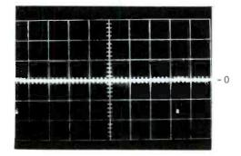
Vertical Trigger, Terminal Q 5 Volts/cm Sweep: 2 msec/cm
