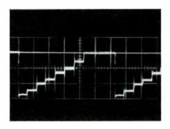
Delay Line Input at Junction of 1R29 and 1R31 1 Volt/CM
