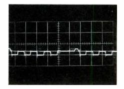
Blue Signal at Kinescope Pin #13 100 Volts/CM Zero Volts DC at Bottom Line of Graticle Zero Volts Reference at Bottom Line of Graticle
