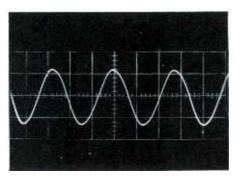
Subcarrier Signal at Point BG or BH 10 Volts/CM Sweep Speed = 1/10 Microsecond/CM
