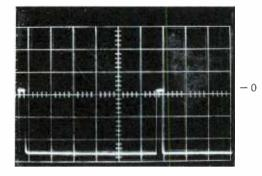
Burst Key Pulse at Terminal AF 5 Volts/cm
