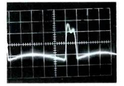
Terminal "A" of Flyback, 5T3 200 Volts/cm Sweep: 10 microsec/cm
