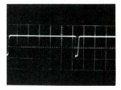
Clamp Pulse at Pin 1 of 4V3 50 Volts/cm Sweep: 10 microsec/cm
