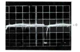
Composite Sync, Terminal N 5 Volts/cm Sweep: 10 microsec/cm
