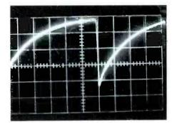
Grid Drive at Pin 5 of 5V4 50 Volts/cm Sweep: 10 microsec/cm
