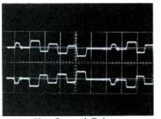
Hue Control Pulses Top Trace Point BM (B-Y) Bottom Trace Point BO (Y-B) l Volt/CM
