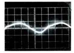
Damper Plate, Pin 2 of 5V7 50 Volts/cm Sweep: 10 microsec/cm
