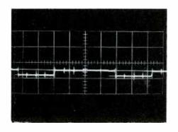
Green Signal at Kinescope Pin #5 100 Volts/CM
