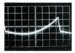
Vertical Convergence at Pin 3 of 5V1 5 Volts/cm; Zero at Bottom of Graticle Sweep: 2 msec/cm
