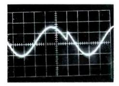
Ringing Coil Voltage at Pin 8 of 5V3 20 Volts/cm Sweep: 10 microsec/cm
