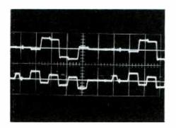
Top Trace: R-Y Signal at Point R Bottom Trace: B-Y Signal at Point S .5 Volt/CM
