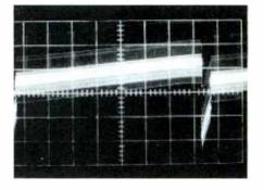
Yoke Voltage at Yellow Lead of 5T1 20 Volts/cm Sweep: 2 msec/cm
