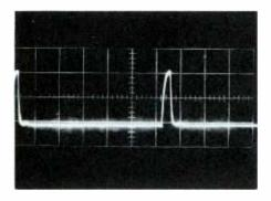
Clamp Pulse at Pin 6 of 4V3 20 Volts/cm Sweep: 10 microsec/cm
