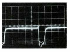
Blanking at Kinescope Grid #1 20 Volts/cm Sweep: 10 microsec/cm
