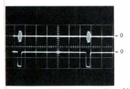
Top Trace: Demodulated Burst at Emitter of 2Q7 2 Volts/CM
